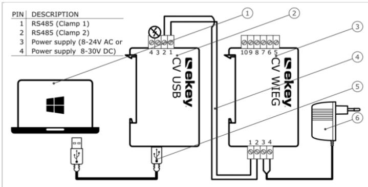
Fig. 6: Wiring diagram for configuring the converter
